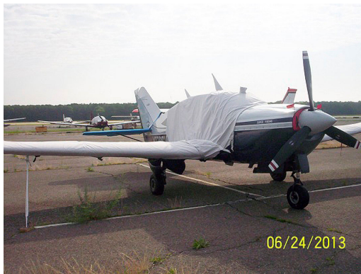
Bellanca Viking Canopy Cover with Wing Root Covers, Wing Covers, Engine Plugs
