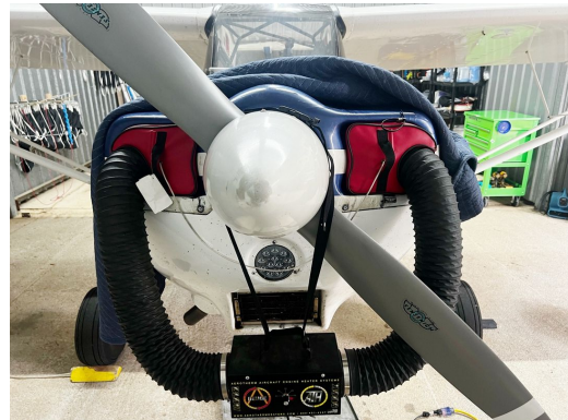
Citabria Engine Inlet Plugs with Aerotherm heater hose cutouts.
