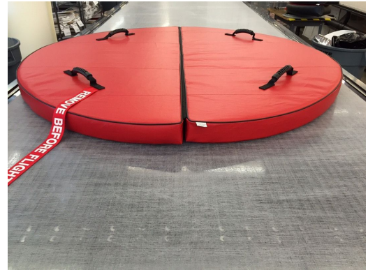
Boeing 737 Max Intake Plug, folding type
