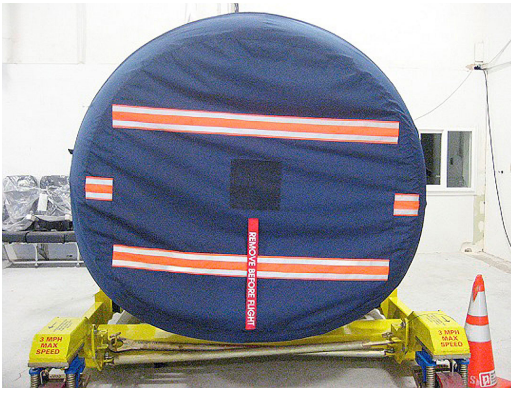
Boeing 737 NG Intake Cover (Installed on CFM56-7BE QEC Engine) Boeing 737 Intake Cover, CFM LEAP-1B (MAX 7, 8, 9 & 10)
