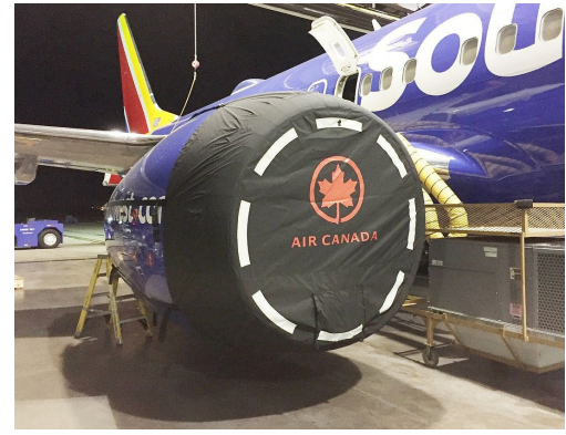
Boeing 737 NG Intake Cover (Installed on CFM56-7BE QEC Engine) Boeing 737 Intake Cover, CFM LEAP-1B (MAX 7, 8, 9 & 10)
