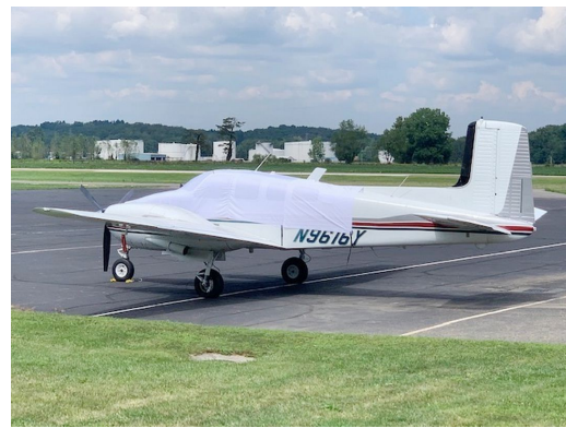
Beech Twin Bonanza Canopy/Nose Cover, test fit cover
