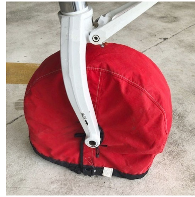
Beech King Air 300 Tire Covers (nose gear)
