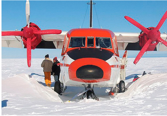
Casa 212 Insulated Engine & Propellor/Spinner Covers
