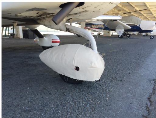
Grumman AA5 Nose Wheelpant Cover, test fit
