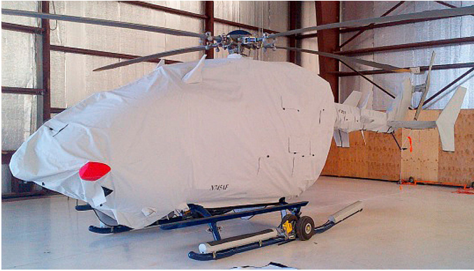
Main Body (also covers bottom), Tailboom, Vertical Pylon, Stabilizers and Tail Rotor Covers
