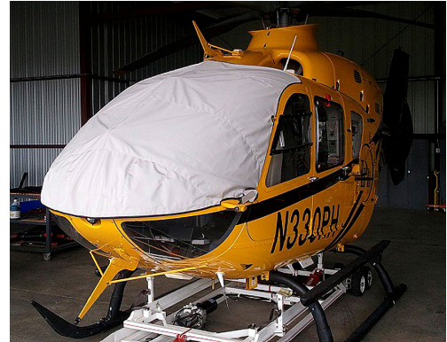
EC-135 Windshield/Skylights Cover, pinches in door jambs
