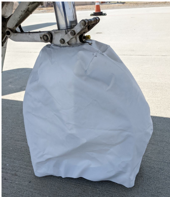
CJ1 Nose Gear Tire Cover, test fit
