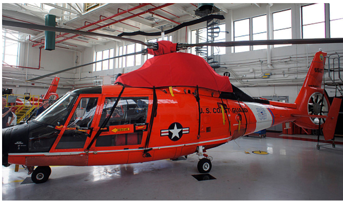
MH-65C Rotor Hub, Swash Plate Aperture, Engine Area Cover set, P/N: A365-210 MH-65C Engine Area Cover, Swash Plate Aperture, Rotor Hub cover set, P/N: A365-210
