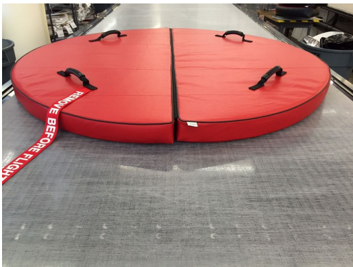
Boeing 737 Max Intake Plug, folding type
