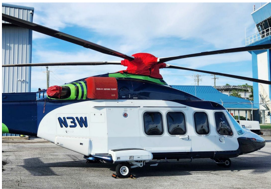
Agusta AW139 Rotor Mast Cover, covers upper deck & aft of rotor mast area
