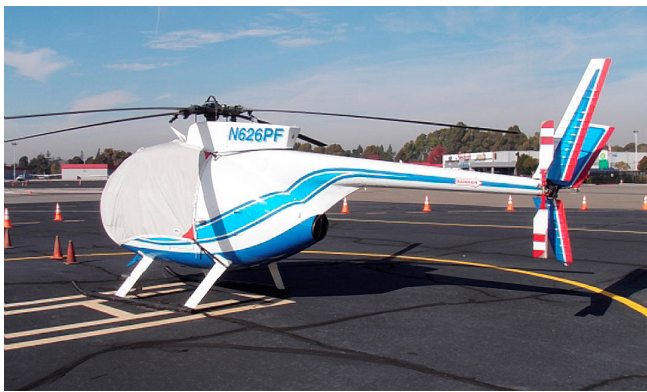
MD500C Bubble Cover with Wire Strike detail
