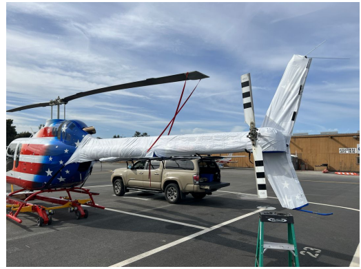
Bell 505 Tailboom & Stabilizer Covers, test fit cover
