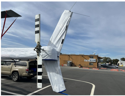
Bell 505 Tailboom & Stabilizer Covers, test fit cover
