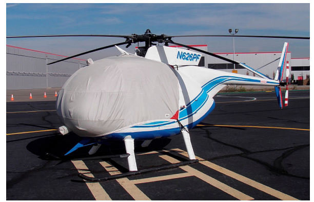
MD500C Bubble Cover with Wire Strike detail
