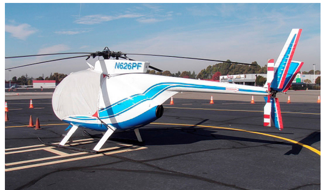
MD500C Bubble Cover with Wire Strike detail
