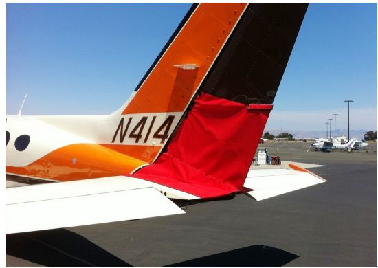
Cessna 414 Rudder Openings Cover (bird barrier)
