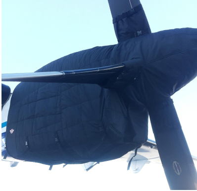
ATR-72-202 Insulated Engine & Prop Hub Covers
