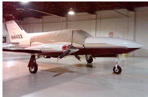
Cessna 414 Canopy Cover and Engine Inlet Plugs
