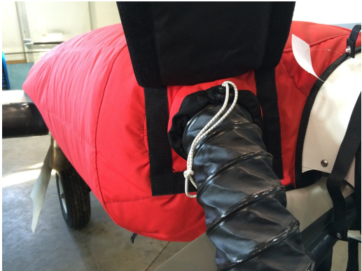
Cessna 402 Insulated Engine Cover with Heater
