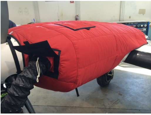
Cessna 402 Insulated Engine Cover with Heater
