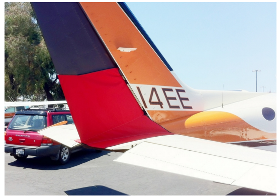
Cessna 414 Rudder Openings Cover (bird barrier)
