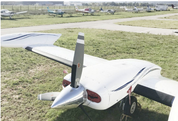
Cessna 340 Engine Inlet Plugs
