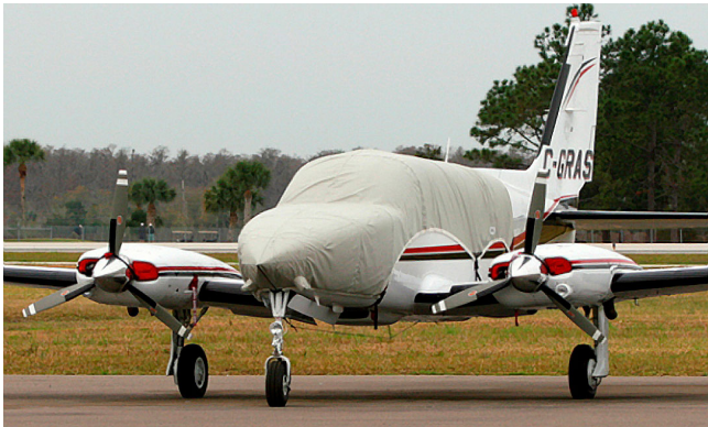
Cessna 340 Canopy/Nose Cover & Engine Inlet Plugs
