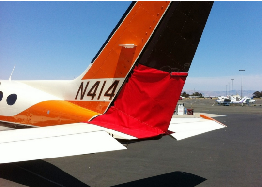
Cessna 414 Rudder Openings Cover (bird barrier)
