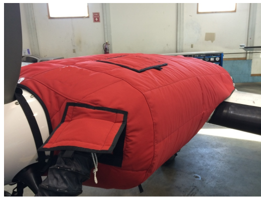
Cessna 402 Insulated Engine Cover with Heater
