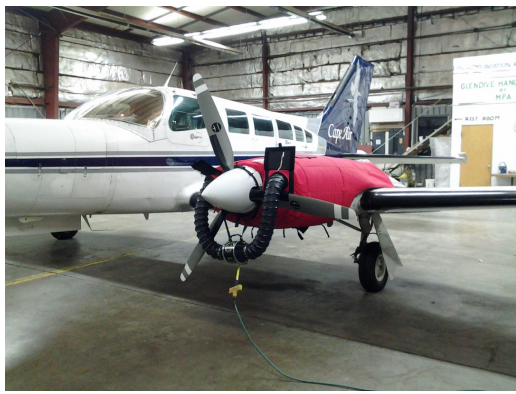
Cessna 402 Insulated Engine Cover with Heater
