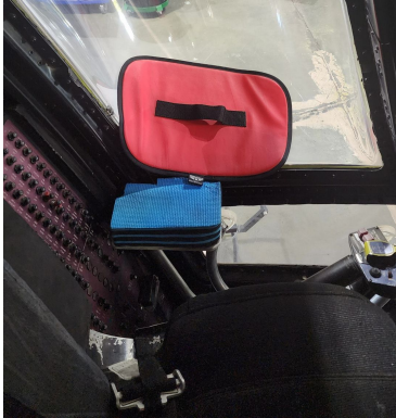
Boeing Vertol CH-47 Logger Window Plug
