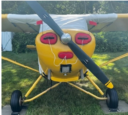
Aeronca 11CC Super Chief Engine Plugs, Extended Canopy Cover (also covers gas caps)
